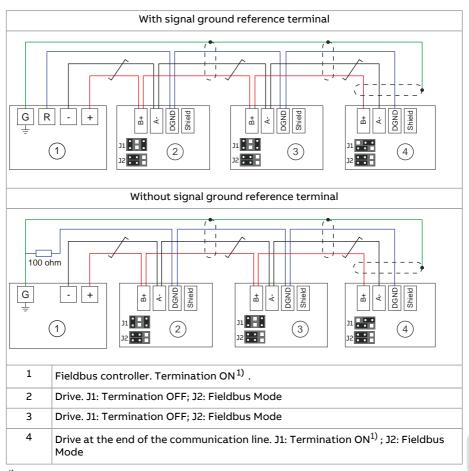
1) Note: The device at both ends on the fieldbus must have termination set to ON.
