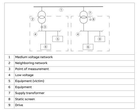
and cables is sufficient. If in doubt, the supply transformer with static screening between the primary and secondary windings can be used.
