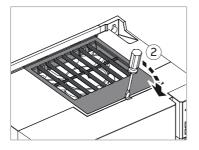
3. Carefully lift the fan cover out of the drive. The fan cover holds the cooling fan.
