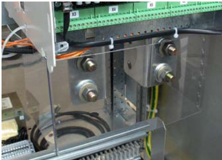
Examples for DC main terminal covers for D3 (left) and D4 (right) converter modules.
